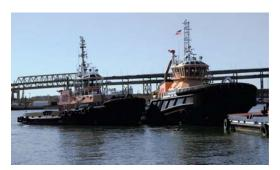
MTU Series 4000 engines are being used to power new Boston Towing and Transportation tugboats used at major LNG terminals along the East Coast.
